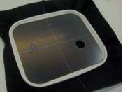
Tighten the set screw to complete the hooping. Note: The fabric should be taut and smooth in the hoop but it should not be pulled or stretched tightly. You do not need to "bounce a quarter" off the hooped fabric as that will cause it to pucker around the stitched design once it is released from the hoop.
