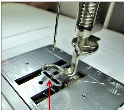
Presser foot lifter is DOWN but the sole of the foot does not touch the machine so you can move the fabric.
