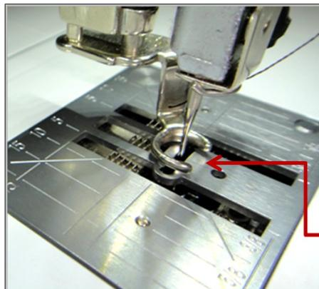
As you take a stitch, the sole of the foot goes down to hold the fabric in place as the needle pulls away
