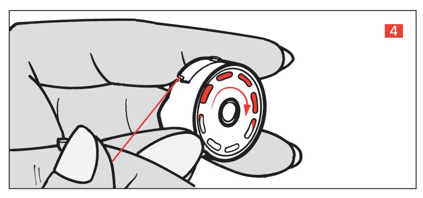
Pull the thread right through under the spring into the T-shaped opening.
