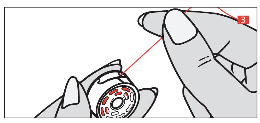
Pull the thread through the slot in the bobbin case.
