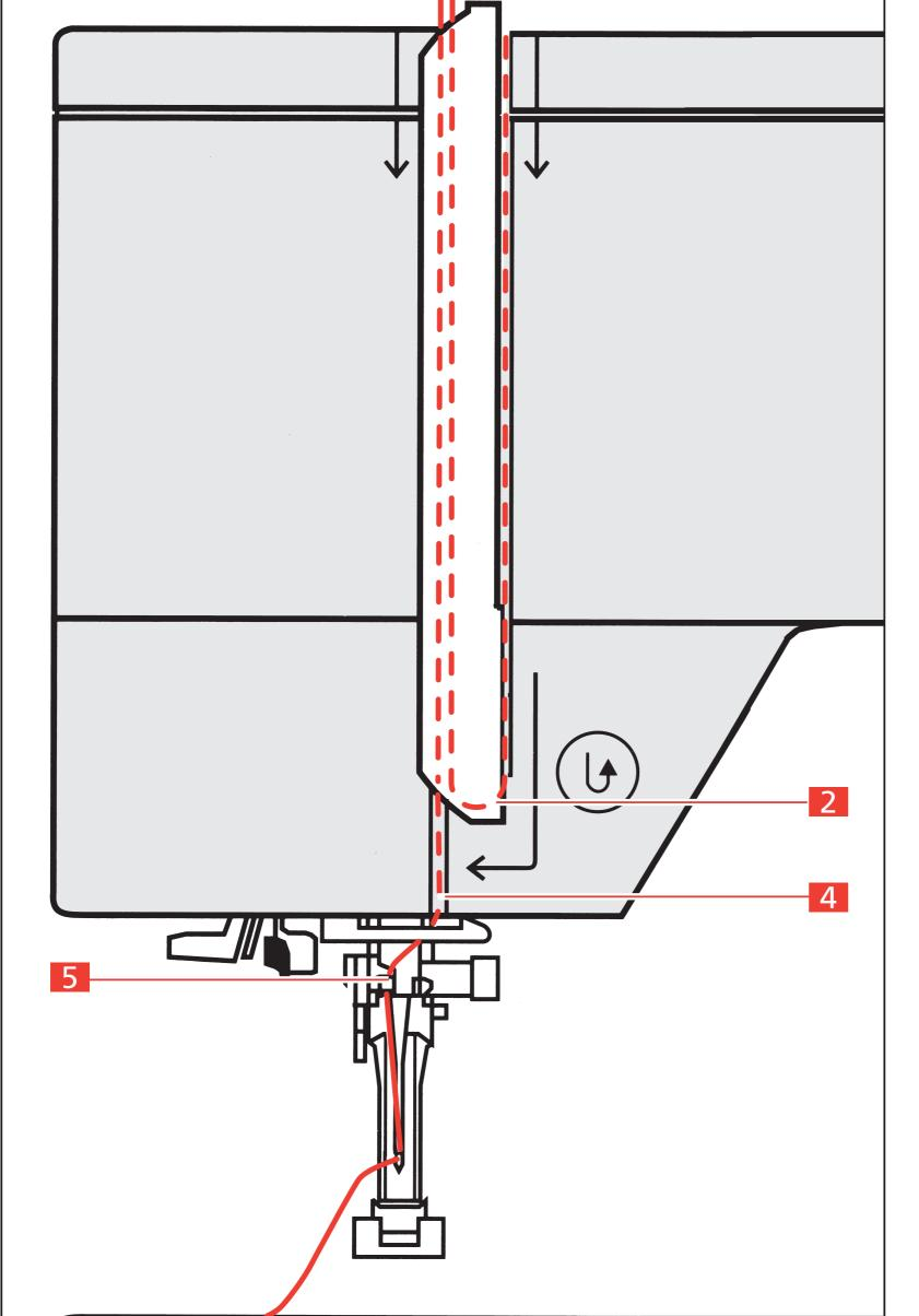
cover to point **2**, then up on the left and into the slot on the take-up lever 3.
