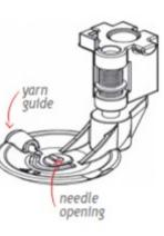
hole in the center of the foot. This places the cord under the needle where it is straight stitched in place.
