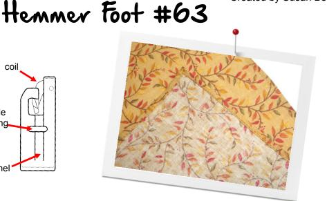
Tip: Use the FHS (Freehand System) to raise and lower the presser foot as you move through the steps below. This keeps both hands free to manage the fabric feeding through the hemmer foot.
