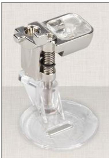
This spring-loaded presser foot is designed to work with the hopper mechanism of BERNINA sewing machines for free-motion stitching. The clear acrylic sole offers visibility of the stitching area and the large size compresses the area around the needle to add to the visibility.
