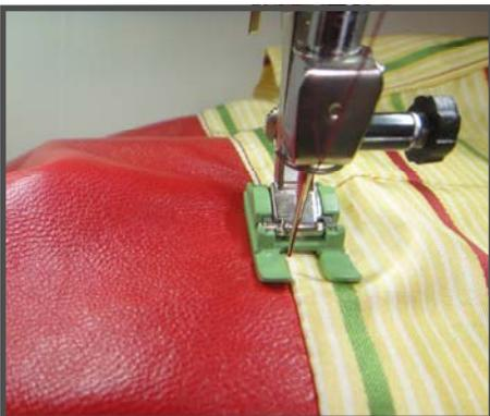
Turn the lining to the inside of the purse, folding 4" of the leather to the inside (this places the magnetic closure on the inside of the purse). Slip the purse over the freearm. Adjust the needle 1-2 positions to the right.
