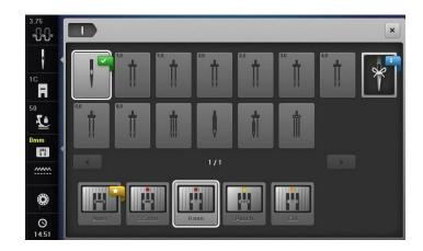
Select the Quilt Menu on the sewing machine (if available). There are several straight stitches located in this menu. Select straight stitch #1326. This has been setup in the machine as the perfect stitch for piecing, at a stitch length of 2.0 mm.
