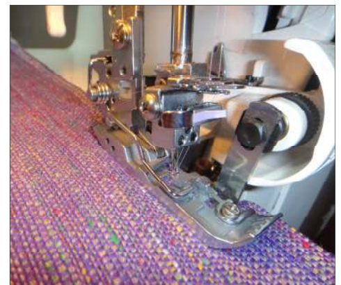
seaming, trimming, and overcasting with one pass under the needle(s)
