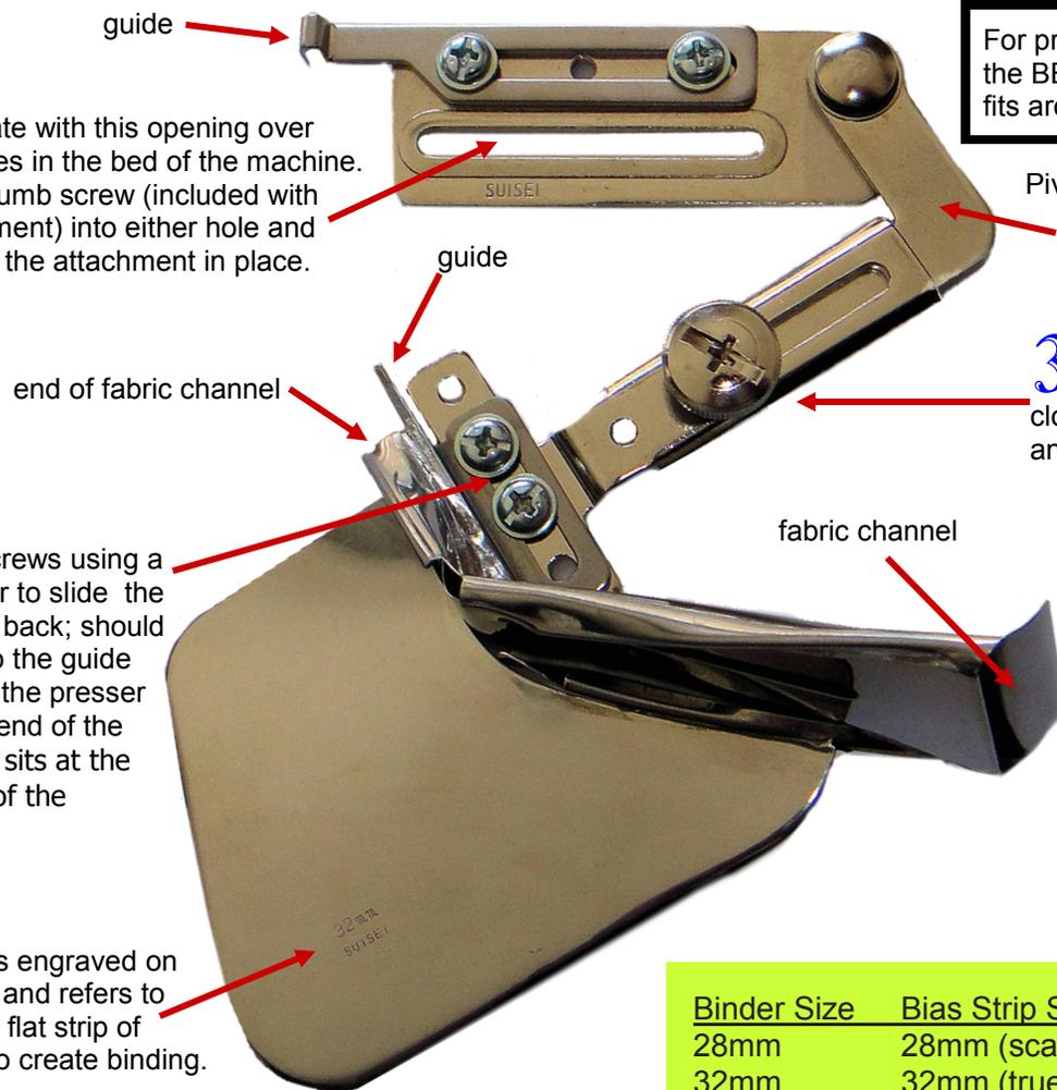
**4** Loosen screws using a screwdriver to slide the binder front to back; should be adjusted so the guide sits parallel to the presser foot while the end of the fabric channel sits at the tip of the toe of the presser foot.
