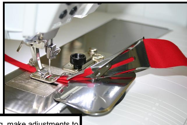
**2** Loosen screws using a screwdriver to slide the guide side-to-side; should be adjusted to fit against the side of the presser foot after the attachment is in place.
