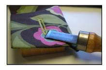
Cut the opening using a Buttonhole Cutter. Place the wooden block under the buttonhole and position the cutter in the slit. Press down to cut through the layers, creating an opening.
