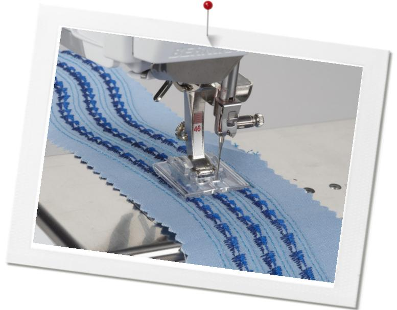
Insert a 3.0mm double needle into the machine and thread with two spools of thread (see right).
