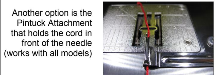
Another option is the Pintuck Attachment that holds the cord in front of the needle (works with all models)
