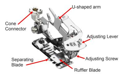
The ruffler moves up and down with the needle bar as the machine is stitching and the ruffler blade moves in and out, pinching small amounts of fabric and pushing them under the needle. The separator blade holds fabric in position, and keeps the ruffler blade from coming in contact with the feed dog of the machine.
