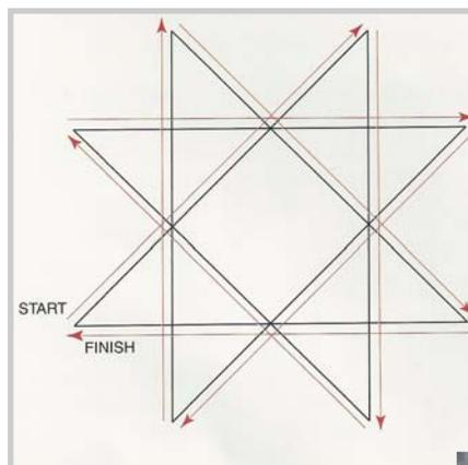
Select the Feather Stitch with default settings. Using Walking Foot #50 with the Center Guide sole, follow the diagram to stitch the star in place.
