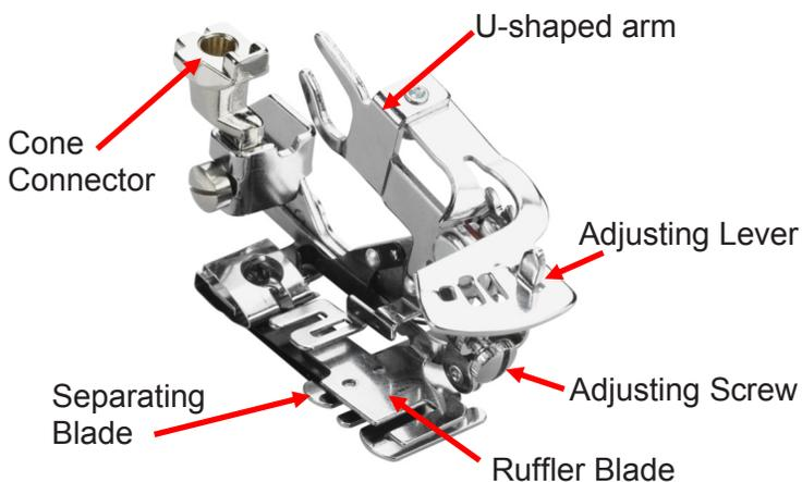
The ruffler moves up and down with the needle bar as the machine is stitching and the ruffler blade moves in and out, pinching small amounts of fabric and pushing them under the needle. The separator blade holds fabric in position, and keeps the ruffler blade from coming in contact with the feed dog of the machine.
