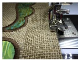
• Using the Edgestitch Foot #10 and the #6 Triple Stitch with a stitch length = 4.5 and Needle position 4, stitch around the top, sides and bottom of the flag.
