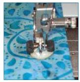
stitch width as needed to match the button holes. Slowly complete the stitch program using the foot control. When done, use the Auto Thread Cutter to trim the thread tails.
