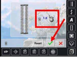
When the slit size is increased, the bead size is automatically reduced. Watch it change as you adjust the slit width. Adjust the bead width to 4.2mm; this will not interfere with the slit width.
