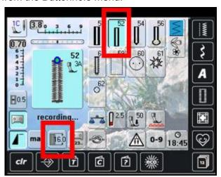
Touch the Buttonhole Length/Measurement icon. Hold your button up to the left side of the screen and use the stitch length or stitch width knob to move the vertical line until it reaches the right side of your button.
