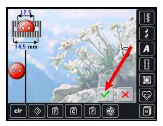
Notice that the measurements on the graphic change as you move the line. The upper number is the size of the button; the lower one is the size of the buttonhole. 2mm is automatically added to the length to allow for the thickness of the button.
