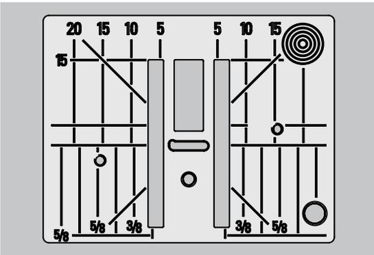
Due to the width of the stitch plate hole the outer feed dog rows are relatively far apart.
