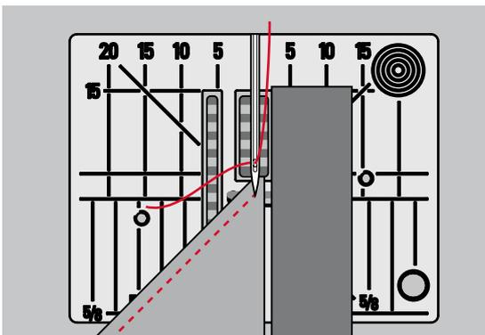
When sewing corners only a small section of the fabric is actually on the feed dog. Therefore it cannot grip the fabric well.
