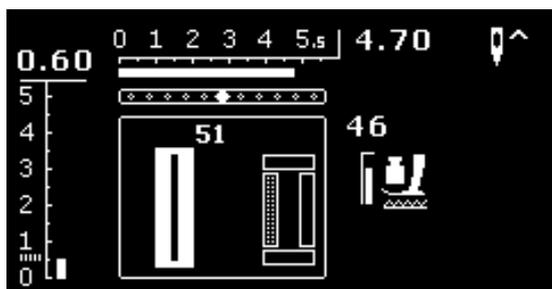
When beginning to sew the actual sequence of the buttonhole is displayed instead of the presser foot indicator.
