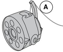
**Thread tension for sewing buttonholes**
