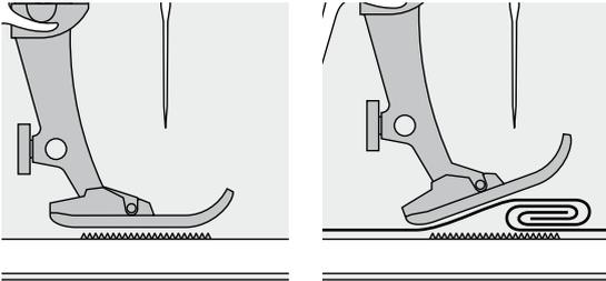
The feed dog works accurately when the foot is level.
