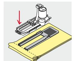
When sewing a buttonhole in difficult materials, we recommend to use the Compensation plate for buttonholes (optional accessory). It can be used along with buttonhole foot with slide No. 3A.
