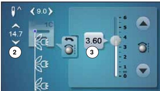
With other stitch patterns, including alphabets, the overall length of a stitch pattern **2** is displayed. The actual stitch length **3** is visible when the stitch length Display is opened.
