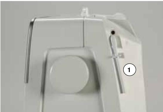
The vertical spool pin is on the side behind the handwheel.
