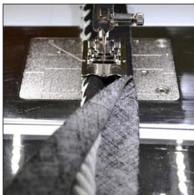
Double Cord Foot #60/60C is heavy and balanced so the fabric does not shift.
