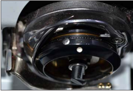
Loosened tension on the BERNINA 8 Series bobbin basket.
