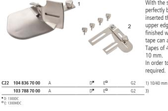
With the single fold binder, fabric edges and necklines can be perfectly bordered with bias tape. The unfolded tape is inserted through the attached guide rail, folded over along the upper edge while the under edge remains open, and is then finished with a cover stitch. For the personalized look, the bias tape can also be cut by yourself.
