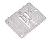
This Stitch Plate has a purple marking and a reduced stitch hole width of 5.5 mm. It fits all 9-mm machines and achieves particularly good sewing results when sewing thin or soft fabrics. All zigzag and decorative stitches up to a width of 5.5 mm can be used to create detailed sewing projects.
