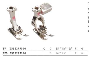
This patchwork foot is ideal for creating beautiful quilts and other precision sewing work. The markings on the sole for seam allowances of 3 mm (1/8"), 6 mm ( $\frac{1}{4}$ ") and 7.5 mm (3/10") ensure accurate guiding. The contact area of this foot is perfect for machines with a 9-mm stitch width, and enables careful guiding of the fabric and stitching when joining pieces of fabric together.
