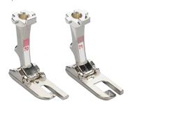
This foot enables precise lap seams to be produced. Since both seam allowances are enclosed and stitched securely in the hem seam, the foot is also suitable for sewing reversible clothing. Foot #70 is suitable for lap seams up to 3 mm wide, whilst foot #71 is suitable for lap seams up to 6 mm in width.
