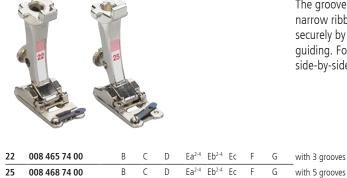
The grooves allow several strands of side-by-side yarns or narrow ribbons to be couched simultaneously, held in place securely by the latch. This means that the yarns do not need guiding. Foot #22 is designed for three and foot #25 for five side-by-side yarns.
