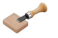
Measuring 1.3 mm ( $\frac{1}{2}$ ") in width, this buttonhole cutter is used to open up sewn buttonholes.
