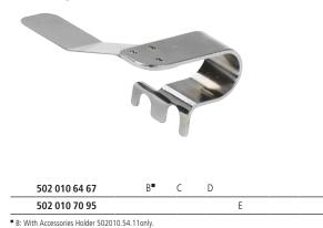
The tab on the attachment separates the two layers of fabric. The bottom layer is gathered whilst the top layer remains flat. You can simply gather a length of fabric, or gather the fabric whilst simultaneously sewing it onto a flat piece of fabric.
