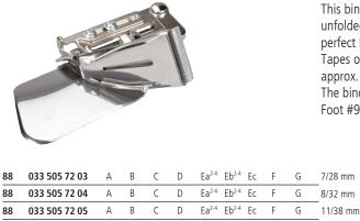
This binder attachment creates perfect edge finishes using unfolded bias tape in widths of 28, 32 or 38 mm. For the perfect look, the bias tape can also be self-made. Tapes of 28, 32 and 38 mm width result in a finished width of approx. 7, 8 and 11 mm. The binder attachment is used in combination with Binder Foot #95/95C.
