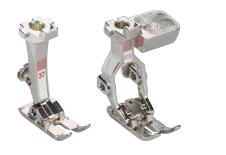
This foot is ideally suited to patchwork projects with seam allowances of 3 mm (1/8/") or 6 mm ( $\frac{1}{4}$ "). The three notches on the side ensure precise guidance for inserting rectangular patchwork pieces.
