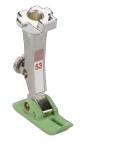
In combination with the straight-stitch plate, this presser foot is ideal for all types of straight-stitching and for narrow seams. Thanks to the non-stick coating on the sole, it passes easily over fabrics that tend to stick during sewing, such as leather and plastics. The two different toe widths serve as guide lines for seam allowances of 3 and 6 mm.
