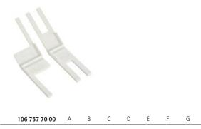
The height compensating tools for overlock or coverstitch make it easy to sew over cross seams and different heights of layers. The heights of 1.5 and 3 mm provide the compensation from finer to thicker overstitching. By sewing on, the height compensation tool is moved away from under the presser foot to the back by means of fabric feed.
