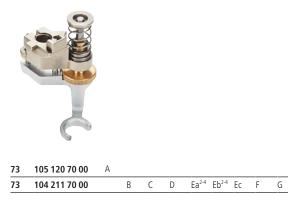
This height-adjustable presser foot is the perfect foot for freemotion quilting and free-motion embroidery. Especially for quilting small patterns and detail work. The open shape of the presser foot sole provides a perfect view of the sewing good. Due to the adjustment wheel, the foot height can be individually adjusted to the fabric thickness. The dull gray coating of the foot prevents the user from being dazzled.
