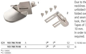
Due to the top bottom double fold binder, fabric edges and necklines can be perfectly bordered with bias tape. The unfolded tape is inserted through the attached guide rail, folded over along the upper and lower edges of the bias tape and sewn on with a cover or chain stitch. For the personalized look, the bias tape can also be cut by yourself.
