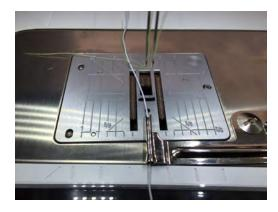
Place pressure foot #1 on the machine. Select straight stitch and increase the stitch length to 3mm.
