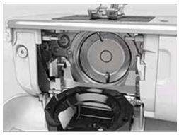
> Fill as much BERNINA-oil into both oil depots so that the felts are damp and make sure that the surface of the hook sleeve (marked in red) remains free of oil.
